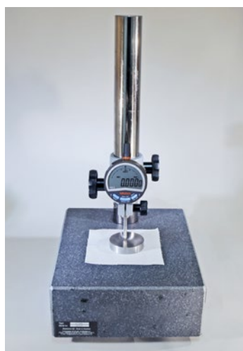
Thickness gauge EV 06 for thickness measurement according to ISO 5084 for textiles.
