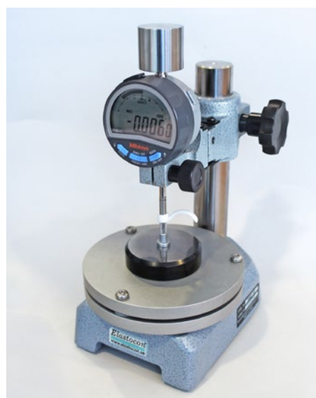
Thickness gauge EV 01 F is a special version, with the possibility to set the parallelity between measuring foot and table.
