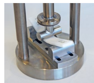
EB 02.29 Fixture for flexural creep by 3-point loading, according to ISO 899-2.
