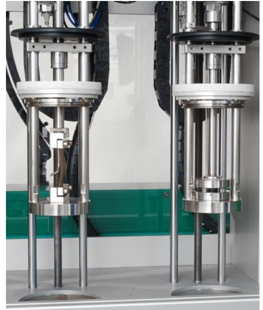
Test stations for testing in tension and for testing in compression.
