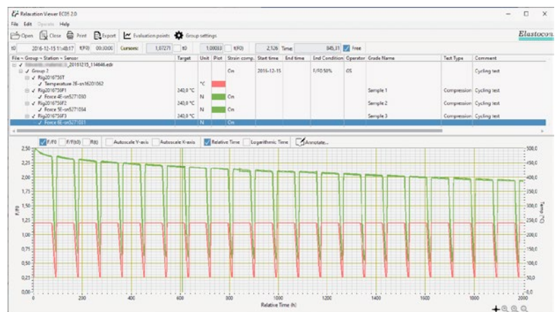
This graph shows a relaxation test with cycling temperature.
