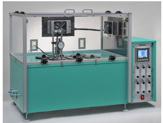
Cell oven 17 for relaxation tests with 6 cells with the same temperature and cycling between subzero to elevated temperature.
