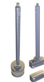
Compression plates and tension grips.
