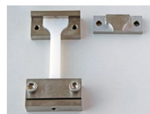
EB 18-II.01 Clamp for creep tests in tension with 50 mm gauge length.
