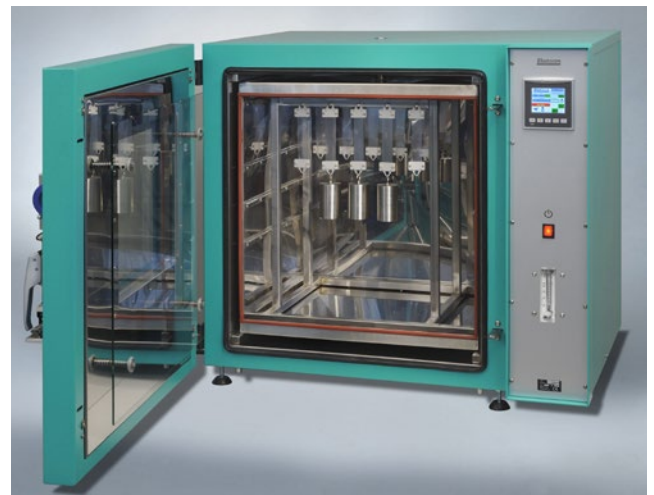
The film creep tester has a fixed set air exchange rate, 7 or 14 changes per hour. It includes hooks to hang 10 test pieces 25 × 100 mm and 10 sets of grips to attach to the test pieces, together with weights, 1,3 kg and 2,3 kg.
