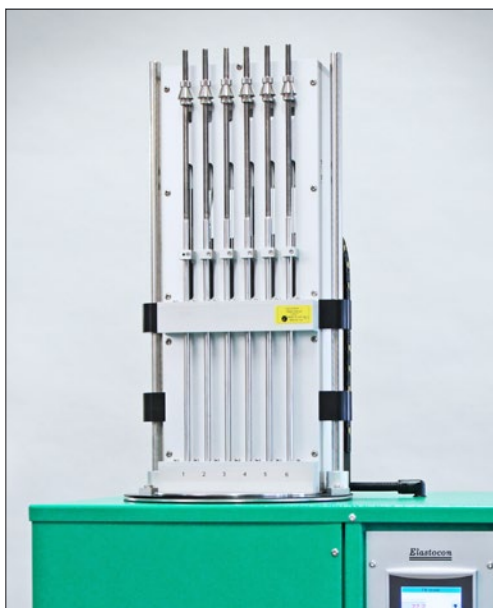
Grips for O-rings (both whole and cut) is an option for the TR Tester.
