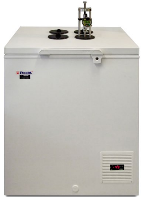
Laboratory Freezer ET 03 with ET03.01 Conversion kit and the EV 09 test rig.
