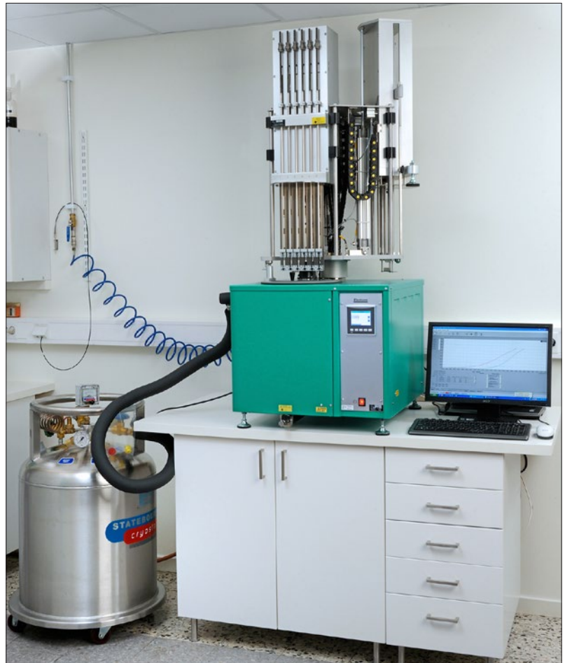
The TR Tester, the Gehman Tester and the Brittleness Tester can be combined using the same base unit with a rig changing system. To the left you can see the automatic cooling with liquid nitrogen, ET 01.02, which consists of both the cryogenic vessel for the storing of liquid nitrogen and the special valve and hose that is needed for the connection between the vessel and the Low Temperature Tester.
