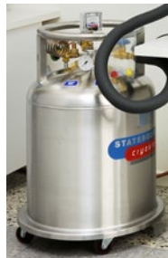
Automatic cooling with liquid nitrogen, ET 01.02.
