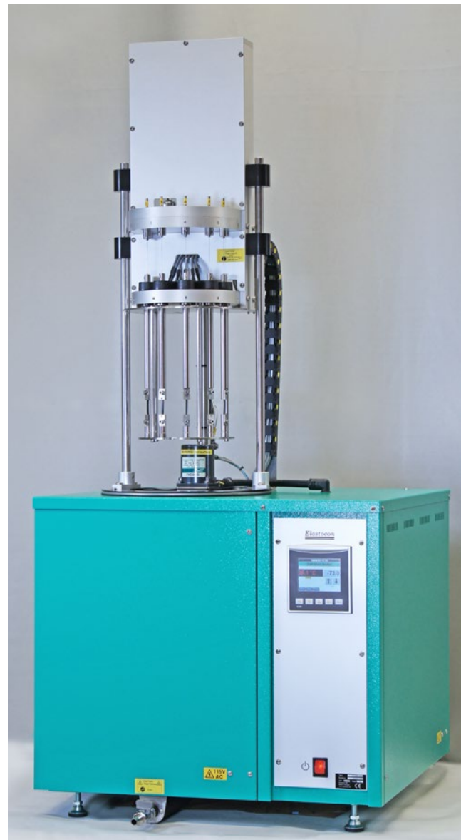
Automatic cooling with liquid nitrogen, ET 01.02.
