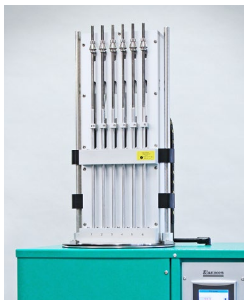
The ET 01.03 grips for O-rings (both whole and cut) are optional for the TR tester.
