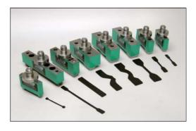
Specimen Cutting Dies, EP 04 are manufactured in both standard and special shapes. A special shank for mounting in presses EP 02 and EP 08 can be fitted. Shanks for other cutting presses are available. All cutting dies are now manufactured with an ejector plate, which helps the work and protects the edges and operator.
