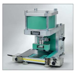
**Specimen Cutting Press, EP 02** for preparation of test specimens of rubber and plastic materials, by punching. EP 02 is a small and compact pneumatic press for preparation of test specimens in the laboratory. EP 02 stands on rubber feet and does not need to be attached to the table.
