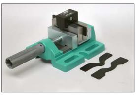
Nick Cutter, EP 07 for making the nick in the test specimen for ISO 34 die B, C and ASTM D624-B.
