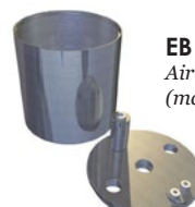
EB 02.01 Container for testing of stress relaxation in compression in liquids.
