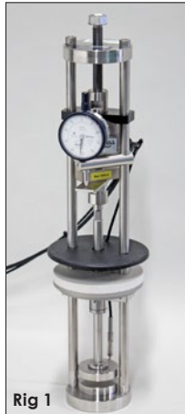
Rig 1 is arranged for testing in compression according to ISO 3384.
