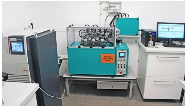
Relaxation system EB 17 with temperature cycling.
