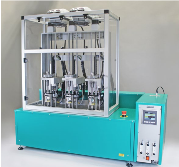
Test stations for testing in tension and for testing in compression.
