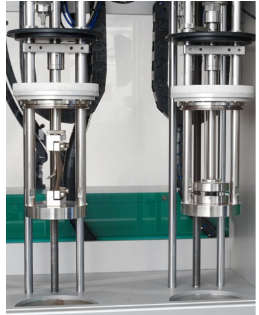
Test stations for testing in tension and for testing in compression.
