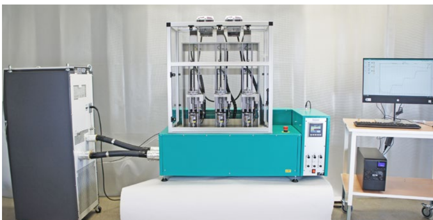
The automatic relaxation and creep tester EB 32 with a liquid circulator for cooling at the left. The EB 32 can cycle between -40 °C and +200 °C, with the same temperature in all test stations.
