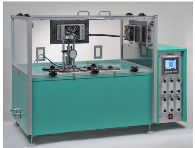
Cell oven 17 for relaxation tests with 6 cells with the same temperature and cycling between subzero to elevated temperature.
