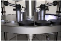
The automatic rotating tray can carry up to 25 pcs of samples. Users can design a test sequence by selecting number of measurements per sample and the desired temperature.
