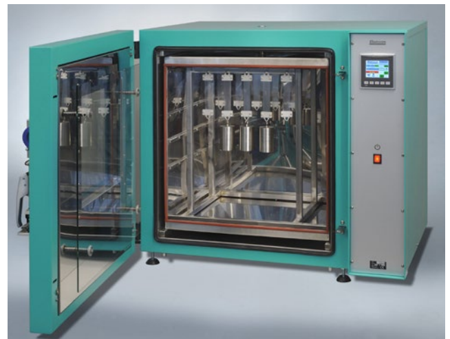
The Film Creep Tester has a fixed set air exchange rate, 7 or 14 changes per hour. It includes hooks to hang 10 test pieces 25 \times 100 mm and 10 sets of grips to attach to the test pieces, together with weights, 1,3 kg and 2,3 kg.
