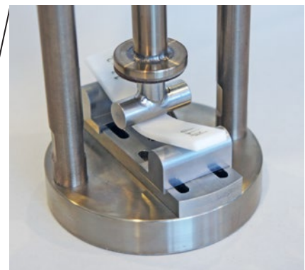
EB 02.29 Fixture for bending test Developed from ISO 899-2.
