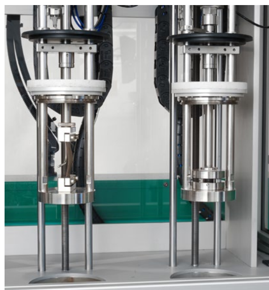
Test station for testing in compression and for testing in tension.
