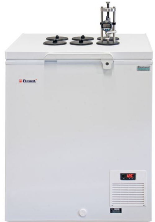
Laboratory Freezer ET 03 with Conversion kit ET 03.01-6 for 6 rigs, and the EV 09 test rig.
