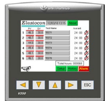
All ageing ovens are controlled from a PLC with a colour touch screen.
