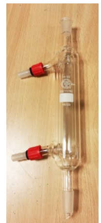
To the right: Option EB 11.04 for the test tube ovens – water cooled condensers when testing volatile liquids.
