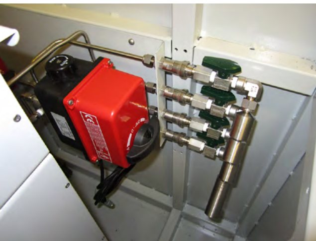
SSU: Upto 4 independent samples collected based on t, T, dT/dt, P, dP/dt
