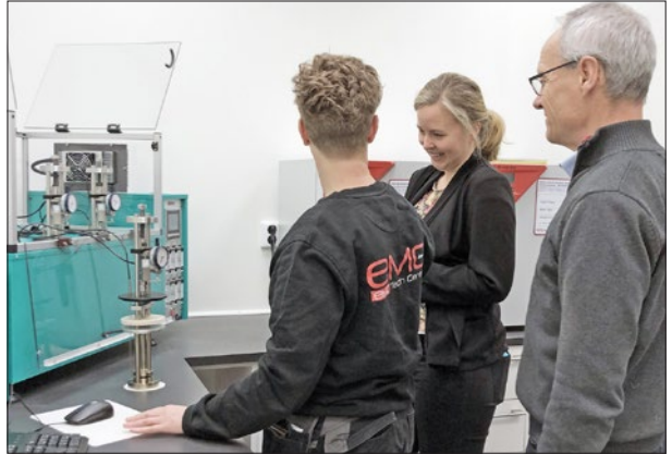
The Relaxation system for continuous measurement of rubber in either compression or tension. It meets the requirements in ISO 3384, ISO 6914 and ASTM D6147.
