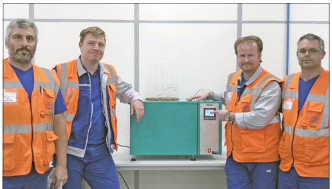
The EB 11-II has 24 test tubes and one temperature. It is used for ageing tests according to ASTM D865 Rubber-Deterioration by Heating in Air (Test Tube Enclosure). The oven can also be used for testing in liquids according to ASTM D471 and ISO 1817 Effect of liquids.
